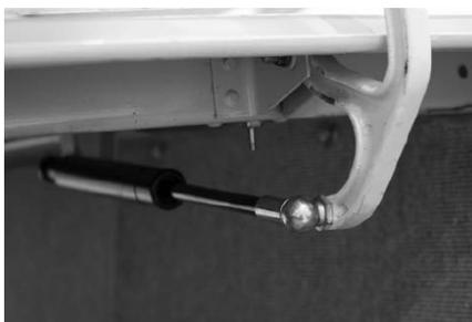
\*Hydraulic actuator detail of the door from front Winery as well mirco-switch that provides close signal and automatically turns off the light.
