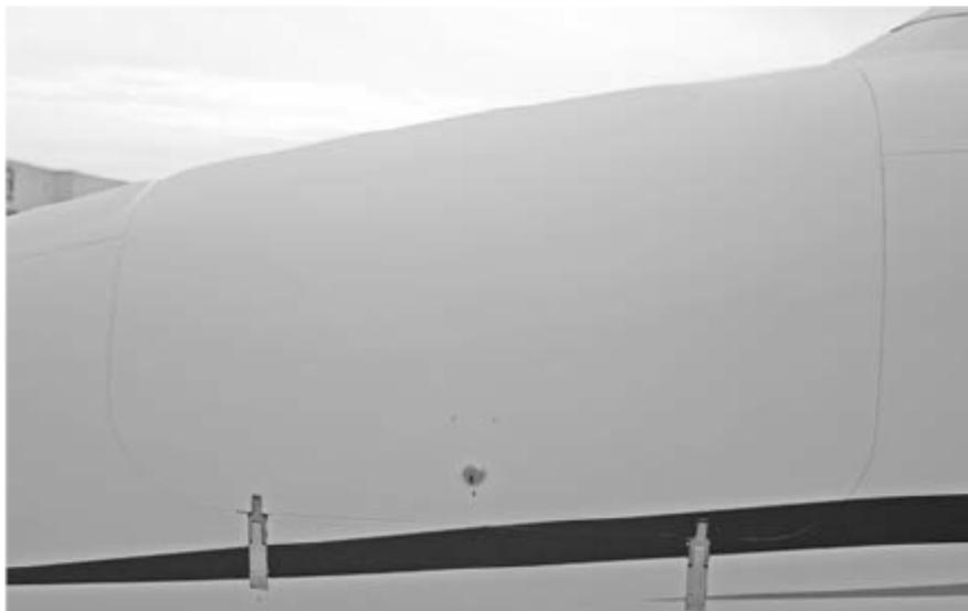
\*Front hold image access (left) door. Right door is symmetrically identical.
