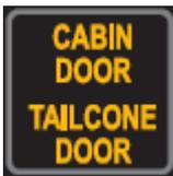
\*Cockpit indicator that the back hold door is open. (Indication shares the same "pill" that the indication that the main access to the plane door is open.
